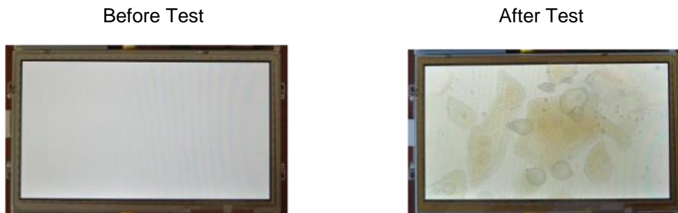
Figure 1. LCD with touch screen irradiated by UV rays in UV irradiation test (Equivalent to 1 year)
