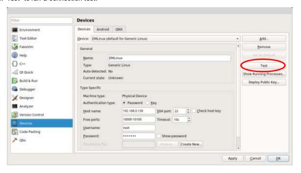
If the connection test is successful, the message "device test finished successfully." will appear.
