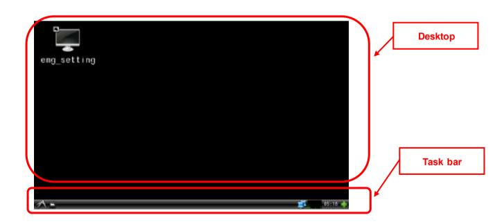
With EM-Linux Auto Start, the items set in "Automatic startup" of the System Setting Tool are executed. The EMG launcher is started by default.
