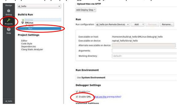
From [Projects] > [Build & Run] > [Build] > [Build Steps], select the [Enable QML debugging and profiling] check box.
