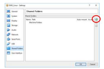
Specify an arbitrary location for the folder path, folder name, and mount point, check the automatic mount, and click the OK button.
